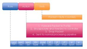
Match Patterns/ Rule: Rule to be constructed from twelve different packet header fields, with various bit widths. The value is computed by the switch based on IP addresses in the packet. In order to predict the same data flow, all the packets make true matching patterns.
