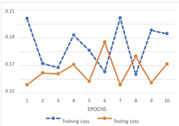
Figure 5 : Representation of the results of training loss, and testing loss obtained by the epochs from the UNSW-NB15 dataset
